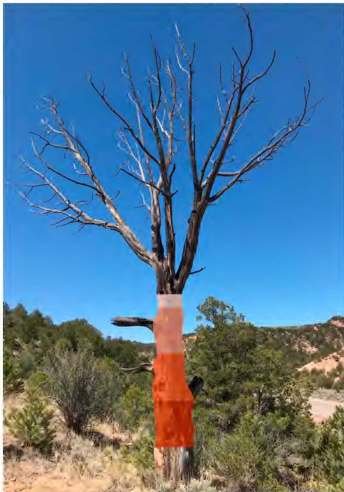
Figure 1. From bottom to top: 30-cm section for steam distillation and analytical analysis (red), 30-cm section for entomology (orange), 30-cm section for fungal and bacterial analysis (pink), 10-cm section for water content analysis (white). Cuts were made in the field using a chainsaw and, as such, are approximations.
